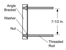
that the posts have to fit inside the mounting clamps (assuming you wish to use the hardware provided by Electro-Mech). The standard clamps form a "pocket" that is 7-1/2 inches square. So, if you try to use a 10-inch diameter pipe, our clamps will not work.
